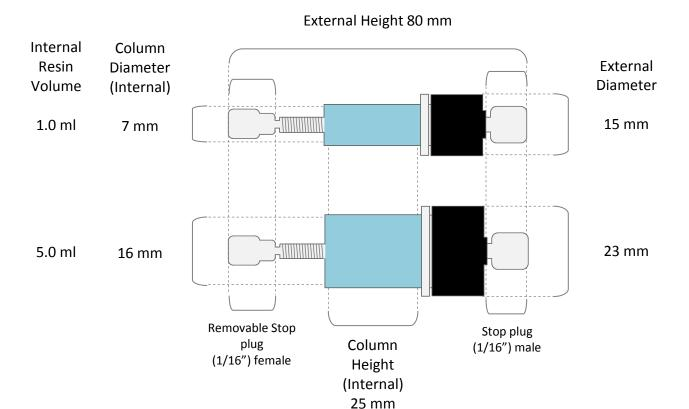
NOTE: HiFliQ FPLC columns are supplied with a moulded removable (1/16") female stop plug attached to the (1/16") male outlet port. Remove prior to use, reverse and use to seal the column for storage.
